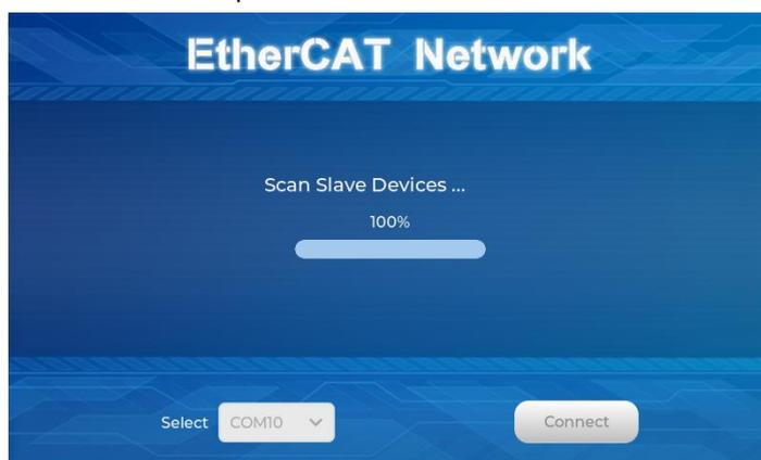
The connected devices will be displayed after the EtherCAT network has been scanned.
