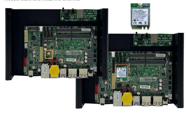
After WLAN/BT module installed, reassemble by the disassembly steps in reverse order.
