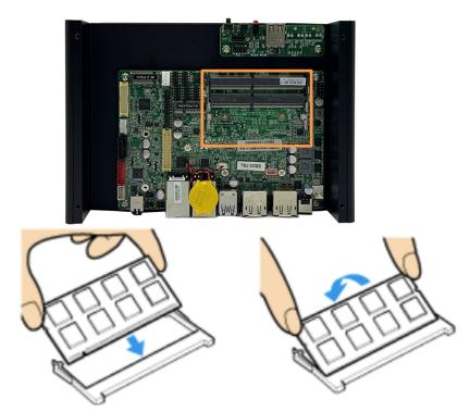
After memory module installed, reassemble by the disassembly steps in reverse order.
