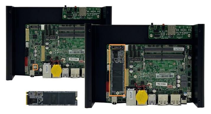
After M.2 SSD installed, reassemble by the disassembly steps in reverse order.
