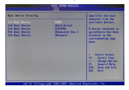
6. Set up the boot device order, press <F10> and select "Save Settings and Exit", press "Y" to save the changes. Unit will restart to the new setup.
