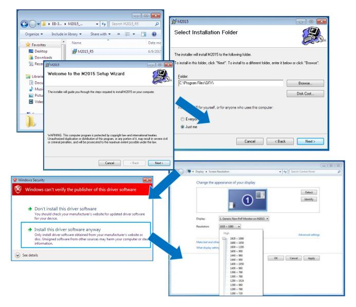
After VGA driver installed, restart computer and you will be able to select resolution up to 1920 x 1080 pixels.
