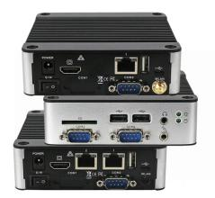
EBOX-IMX8MM Series equipped with an NXP i.MX8M Mini Quad-core 1.6GHz ARM Cortex-A53 processor. Unit supports 1GB to 4GB LPDDR4 of onboard memory, eMMC from 8GB to 64GB onboard, dual COM plus one console ports and a Fanless design.
